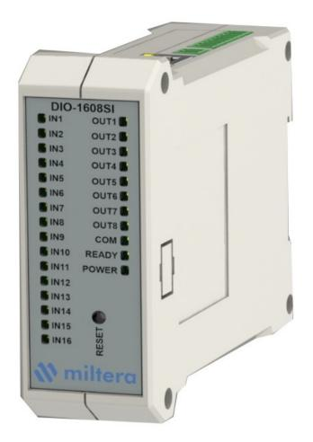
The MTIO modules support the most often-used protocols for retrieving I/O data, making it capable of handling a wide variety of applications. They can be used with Modbus TCP for OT engineering. RESTfull API and MQTT can be used for IIOT platforms.
